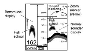
Figure 2-9 Bottom-lock display plus normal sounder display
